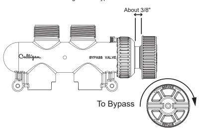
Figure 1. Bypass valve
